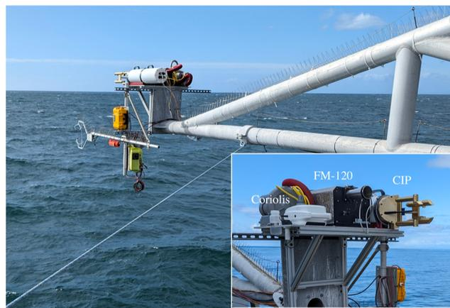
**Figure 1.** Instrument deployment configuration for this study at the SIO Pier end. Instruments were deployed side-by-side (inset) approximately 10 m above mean sea level on a retractable boom arm 6 m away from the SIO Pier structure.
