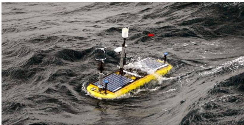
An instrumented Wave Glider during the NSF Pioneer Array experiment in October 2018 prior to recovery after 4 weeks at sea.
