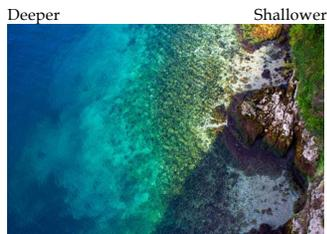
Figure 3: We will incorporate measured bathymetry (LiDAR) into hyperspectral data processing workflow. Constraining the water depth is expected to improve habitat classification, as optical properties change significantly with depth.
