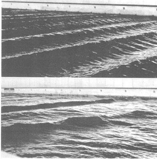
**Fig. 3.** Photographs of progressive wave trains illustrating the wave breaking due to the instability. Upper photograph is made near the wave maker; lower at 60 m from it. The main wave length is 2.2 m. From [6].
