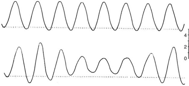
**Fig. 2.** Evolution of a wave train with the main frequency of 0.85 Hz in a water tank. Upper record is taken at a distance of 60 m from the wave maker; lower record is for 120 m. Time marks are at each 0.1 s. Vertical bar is in inches. From [6].
