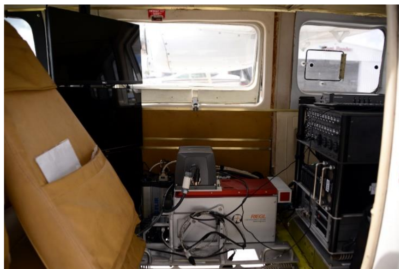
MASS monitor stand (left), instrument package (center) and acquisition rack (right) as installed on a Partenavia P68.
