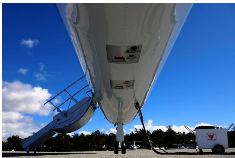
Modified MASS instrument payload packages installed on the underside of a NASA Gulfstream V fuselage.
