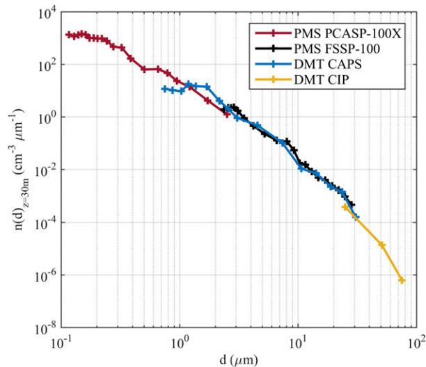
FIG. 4. Representative example of aerosol number distributions taken on 15 Jul 2015 2010 at 2330 UTC during the HIRES experiment, showing the overlap between the four sensors: PMS PCASP-100X (red), DMT CAPS (blue), PMS FSSP-100 (black), and DMT CIP (yellow).
