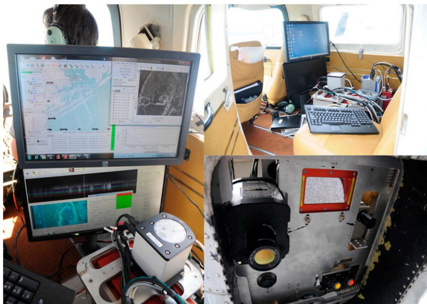
FIG. 2. MASS installed on a Partenavia P.68 aircraft during the RIVET experiment, New River Inlet, in May 2012. (left) Operator in-flight display, (top right) MASS installed in the P.68, and (bottom right) view of MASS from below the aircraft.
