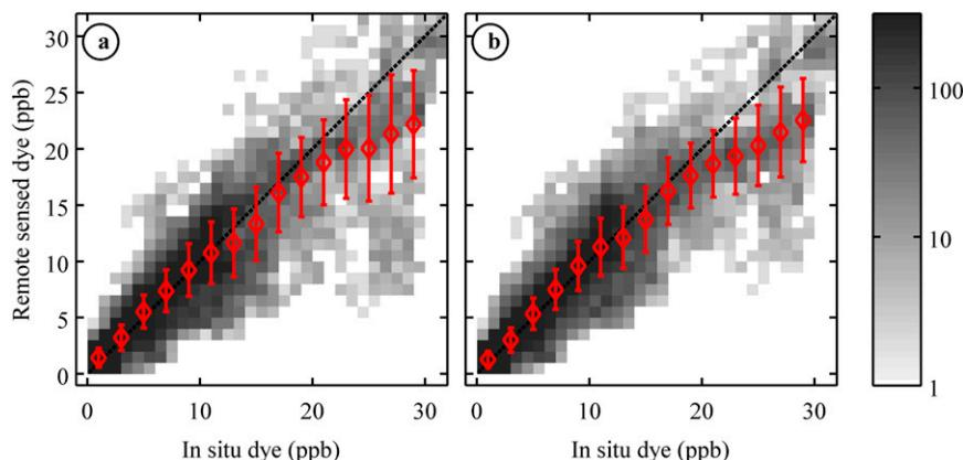
FIG. 7. (a) Hyperspectral dye estimate  $\mathcal{D}_H$  (4) and (b)  $\mathcal{D}_{H4}$  (5) vs in situ-measured dye concentration during RIVET, shown as binned means plus or minus one standard deviation (red curve) and the number of samples (logarithmic gray background, see legend). All data points shown are used in fitting (4) and (5).
