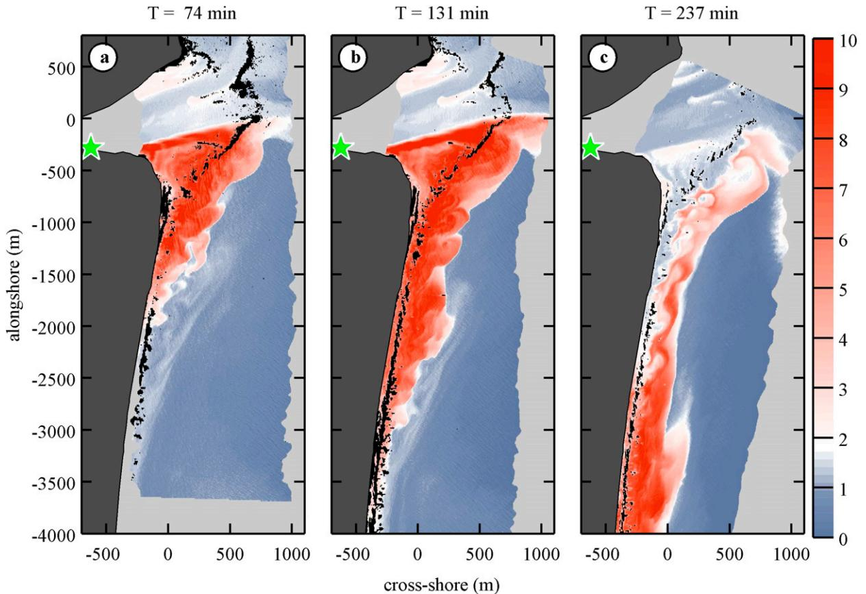
FIG. 8. Hyperspectral estimated dye concentrations (ppb; see legend) on 7 May 2012 during RIVET. Dye was released continuously just inside the inlet (green star symbol) from  $T = 0$  to 139 min, and image times are noted in the panel titles. Dark gray regions indicate land, light gray regions indicate water outside the imaged area, and black regions indicate foam from breaking waves.
