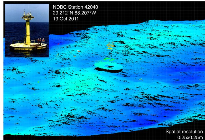
Fig. 2. Example of surface elevation as measured from the MASS during a recent experiment in the Gulf of Mexico, flying above NDBC buoy #42040. (wind~12m/s, Hs = 3.1m)
