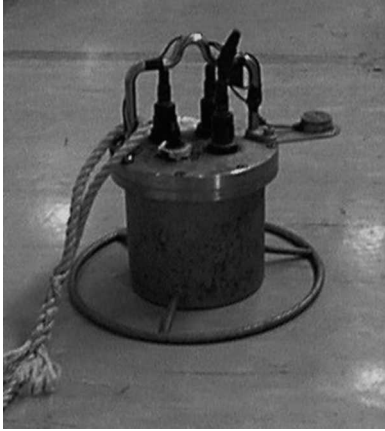
FIG. 8. Subsurface hydrophone housing. The sensing head is seen on the right. On the top of the housing, there are waterproof connectors for the cables.
