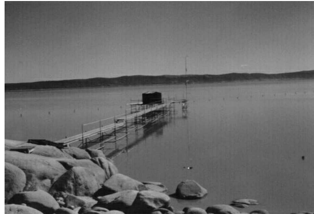
FIG. 2. View of the experimental site with elevated walkway, observational platform with computer shed on it, and suspended measurement bridge. The photo was taken before 1998, when the second anemometer mast was erected away from the bridge.
