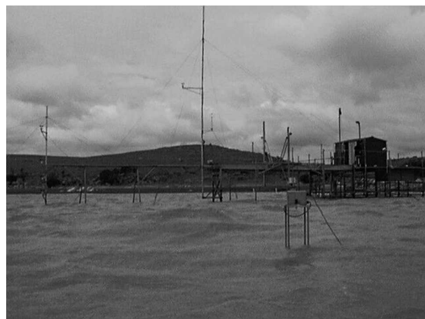
FIG. 3. Offshore view of the experimental site. The platform, computer shed, measurement bridge, and anemometer masts are seen. The device in the foreground is a mobile single-probe wave array.
