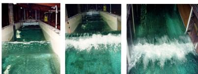
Bubble size distributions are determined by the inversion of broadband (4kHz-100kHz) acoustic signals transmitted between a source and receiver hydrophone pair separated by a fixed pathlength (Terrill 1998, Terrill & Melville 1998). The acoustic technique has been tested beneath laboratory generated breaking waves in seawater using an independent optical bubble sizing technique (Geissler & Jahne 1997) and found to give good results.
