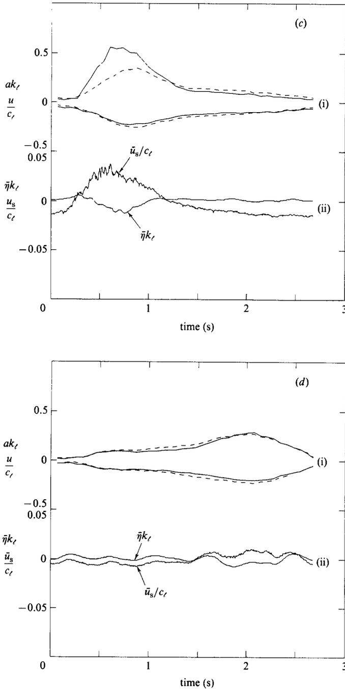
FIGURE 8. (i) Phase-averaged envelopes of surface displacement  $ak_t$  (---) and velocity  $u/c_t$  (—). These were computed by averaging crests and troughs over 100 bins in the period of the wave envelope. (ii) Phase-averaged surface displacement  $\bar{\eta}k_t$ , and velocity  $\bar{u}_s/c_t$ . (a)  $xk_t = 177.1$ ; (b) 193.2; (c) 241.5; (d) 273.7.
