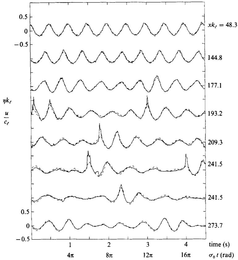
FIGURE 2. Time series of dimensionless horizontal velocity,  $u/c_z$  (—), and surface displacement,  $\eta k_z$  (----), at consecutive stations at distances  $xk_z$  downstream of the wave generator. Here  $c_z$  and  $k_z$  are the linear phase and speed and wavenumber for ( $\sigma_0 = 2$  Hz) deep-water waves, and the initial uniform wave amplitude  $ak = 0.23$ .
