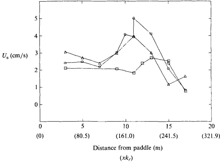
FIGURE 4. Mean surface velocity  $U_s$  as a function of downstream position  $xk_\gamma$ , for  $\square$ ,  $ak = 0.23$ ;  $\triangle$ ,  $0.25$ ;  $\circ$ ,  $0.29$ . Note the local maxima in the region of wave breaking. Mean is a time average over the full record period (13.65 min).
