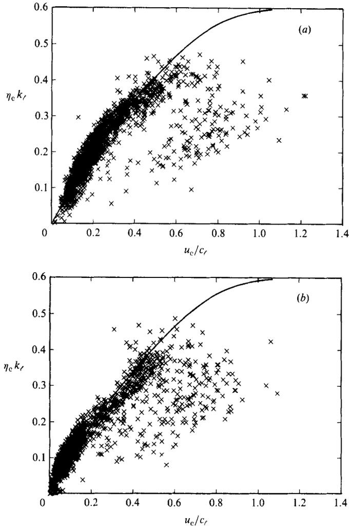
FIGURE 10. Correlation between surface displacement at the crest,  $\eta_c k_\ell$ , and horizontal velocity at the crest,  $u_c/c_\ell$ , for  $ak = 0.23$  at (a)  $xk_\ell = 209.3$ ; (b) 241.5. Also plotted is Cokelet's (1977) numerical prediction of  $\eta_c k$  versus  $u_c/c$ .
