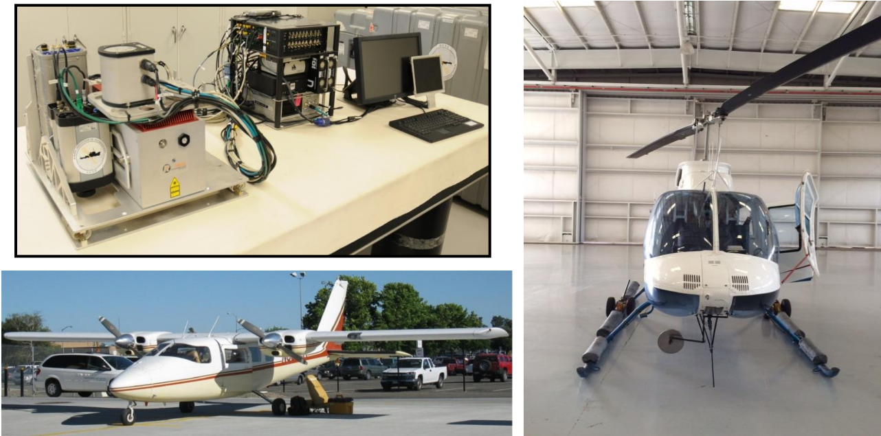
Figure 1. The MASS system on the bench at the Air-Sea Interaction Laboratory, SIO. It is flown on the Partenavia P68 light twin-engined aircraft and the Bell 206 L-III helicopter.
