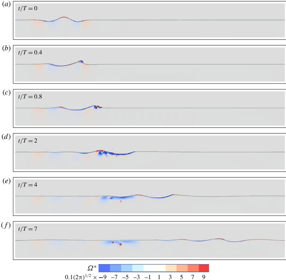
FIGURE 3. Time evolution of a plunging breaker with the vorticity field  $\Omega^* = \Omega/\omega$  at different time steps. The wave starts at the left of the numerical domain, propagates to the right and breaks after half a period of propagation. The waves then propagate out of the region where breaking occurred, leaving an active vorticity field that characterizes the post-breaking flow. The initial conditions were chosen such that  $S = 0.55$ ,  $Re = 4 \times 10^4$ ,  $Bo = 200$ .
