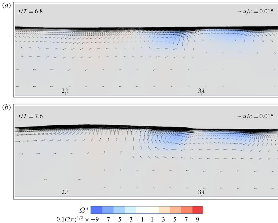
FIGURE 4. The normalized vorticity field  $\Omega^*$  remaining in the region after a plunging breaker, and after the remaining waves have propagated away. The post-breaking flow is characterized by a compact region of vorticity, outside of which the flow is largely irrotational.  $Re = 4 \times 10^4$ ,  $Bo = 200$  and  $S = 0.5$ .
