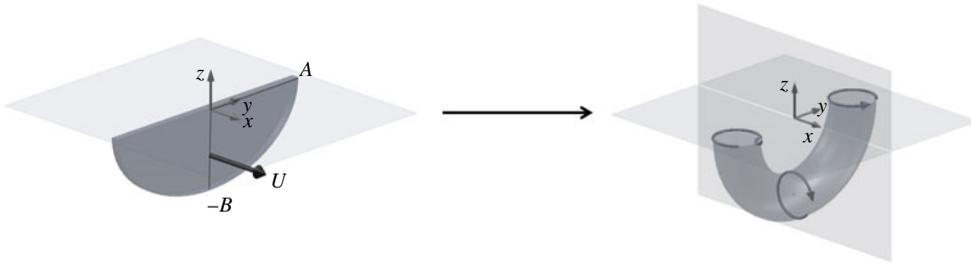
FIGURE 2. A sketch of the bulk scale effects of deep-water breaking on the water column. We assume that breaking acts like a thin impulsively forced disc of semi-major axis  $A$  and semi-minor axis  $B$ , being forced from rest to a speed  $U$  along the  $x$  direction. The disc is then assumed to dissolve, with the flow rolling up where it is strongest, that is along its perimeter, leaving a persistent vortex ring that characterizes the ensemble-averaged post-breaking flow.
