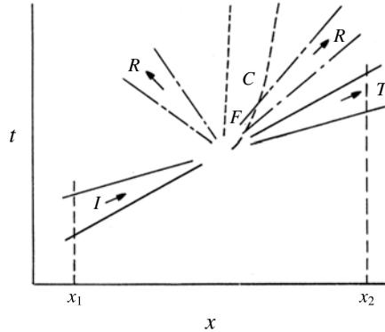
FIGURE 1. A schematic of the focusing wave groups considered in this paper, from Rapp & Melville (1990). The incident wave group,  $I$ , focuses at  $F$ , radiating,  $R$ , and transmitting,  $T$ , waves away from this region. In the area of breaking, currents,  $C$ , and turbulence will be generated. Far upstream and downstream of the breaking region,  $(x_1, x_2)$  respectively, the waves are approximately linear.
