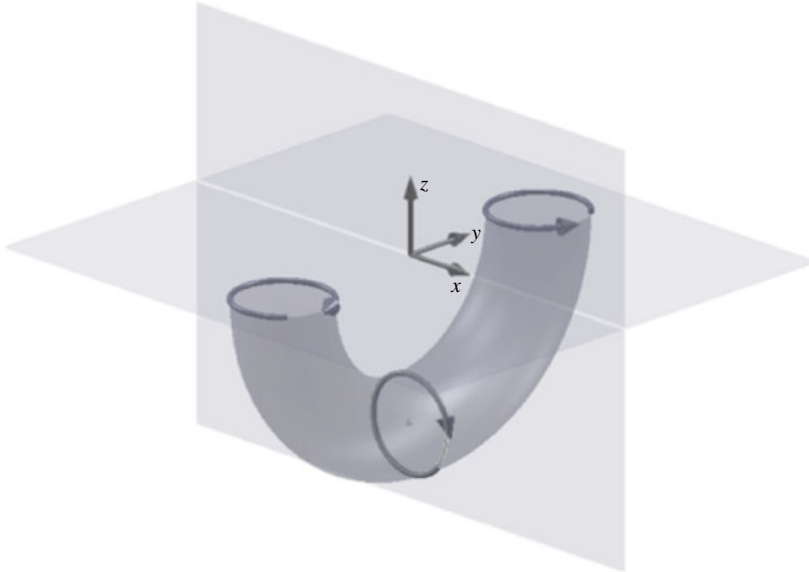
FIGURE 4. Description, proposed by Peregrine (1999), of the topological shape (a half vortex ring) of the flow shortly after a breaking event. The surface of the torus denotes the vortex filament and the arrows indicate the direction of the velocity.
